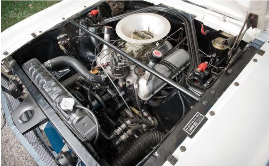
Other special features of the Shelby GT350-R included Tri-Y headers, 34 gallon baffled fuel tank, dual S-W electric fuel pumps, modified steel valve breather covers, competition fiberglass bucket seats, and baffled steel high capacity oil pans. The car's gearbox featured an aluminum case, and the GT350-R was equipped with a protective four-point roll bar. The GT350-R rode on American Racing 15 x 7-inch five-spoke wheels.
