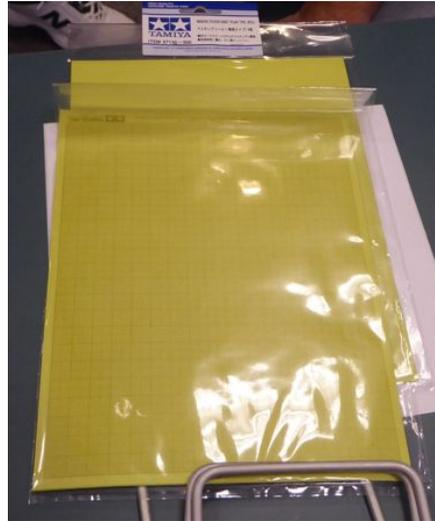
Great masking materials. Avery label sheets are pressure sensitive paper that can be cut as required, and the Tamiya sheets are solid sheets of the Tamiya kabuki tape we are all familiar with. There is also a Tamiya sheet with a grid pattern printed on the surface. Available for office supply stores or on-line.
