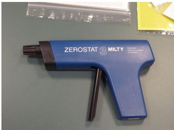
Developed by vinyl record enthusiast to remove static electricity from records. Uses piezo crystal to induce an electric pulse. Not cheap (\$90 -\$100 range), but just the thing to remove that pesky dust inside canopies.
