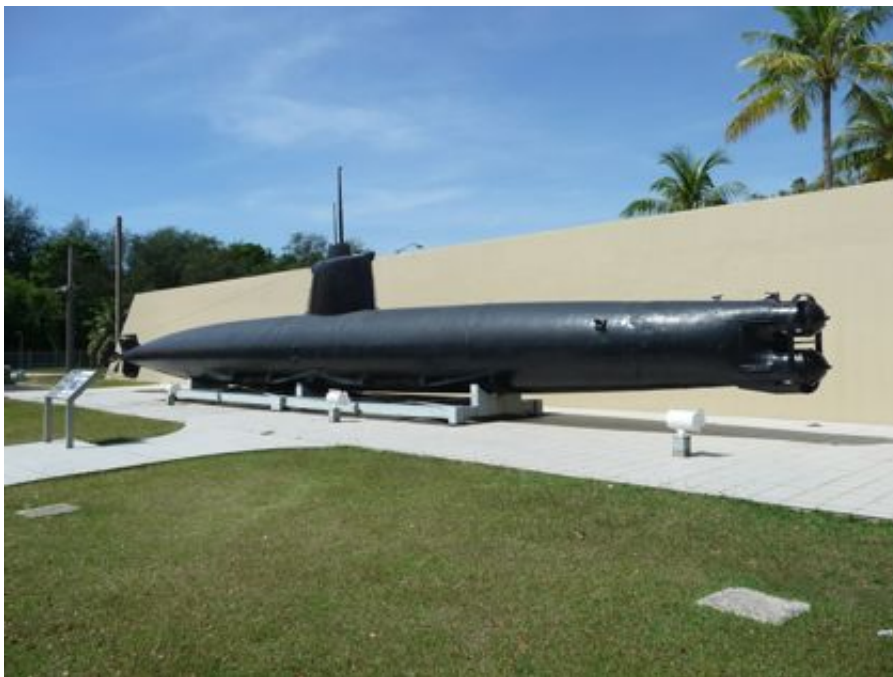
Japanese Ko-hyoteki –class, Type A 2-man midget submarine
