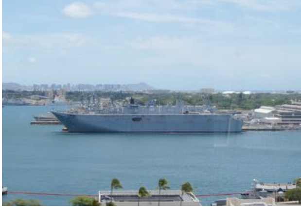
Australian Canberra -class carrier. Similar to a US LHD. Only carries helicopters at this time, but has a 'ski jump' to accommodate STOVL in the future. F-35?
