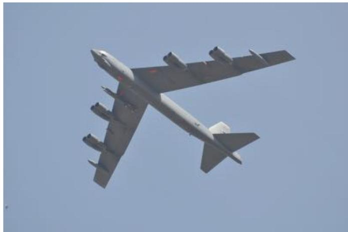
The “Grand Old Lady”, the B-52H. This is 60-031, which is new to Edwards. The configuration is kind of interesting, with a single weapons pylon, and the rarely-seen chaff dispenser pod pylons between the engines, one of which has some sort of orange pod. There are also a number of ‘flight test orange’ panels on the airframe
