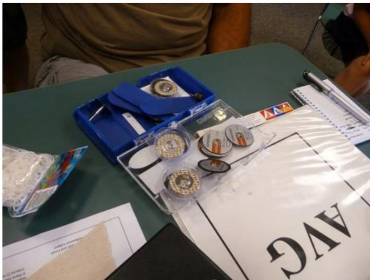
This is a new system from Dremel called EZ-Lock. It has a quick-change feature that allows you change out the wheel on the spindle with just a quick turn, instead of messing with a tiny screw. These are about \$12 to 15 a set at places like Home Depot and Lowe's.
