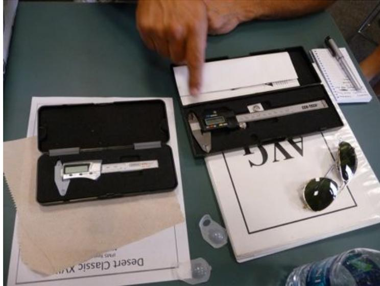
What the heck do I need a set of digital calipers for, you might ask yourself. Well, how about transferring dimensions? Or measuring a rigging span for a biplane. I know you can think of more, and they have uses outside of modeling. The small ones on the left are \$16 from Micro-Mark, while the larger set is \$15 from Harbor Freight. I have a nearly identical set that I use at work and they work great.
