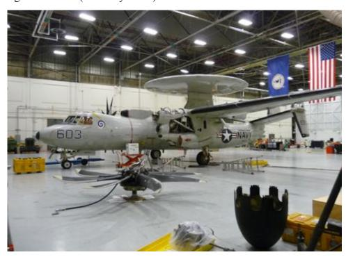
This Hawkeye from VAW-123 "Screwtops" ingested a bird in the No.1 engine while in the pattern and tore up the first stage compressor pretty good. Currently in our hangar for an engine change
