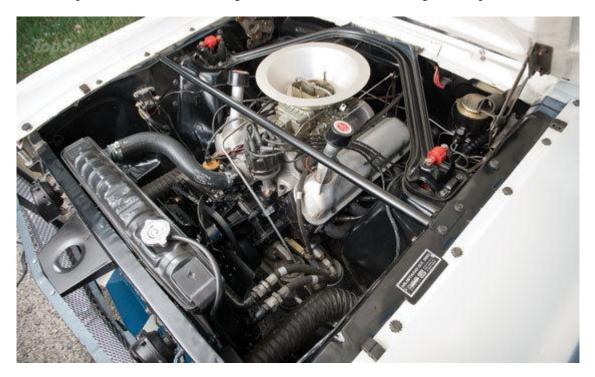
Other special features of the Shelby GT350-R included Tri-Y headers, 34 gallon baffled fuel tank, dual S-W electric fuel pumps, modified steel valve breather covers, competition fiberglass bucket seats, and baffled steel high capacity oil pans. The car's gearbox featured an aluminum case, and the GT350-R was equipped with a protective four-point roll bar. The GT350-R rode on American Racing 15 x 7-inch five-spoke wheels.
