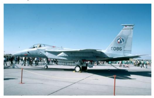
F-15A ASAT. ASAT stood for Anti SATellite, and referred to the ASM-135 missile carried under the fuselage.
