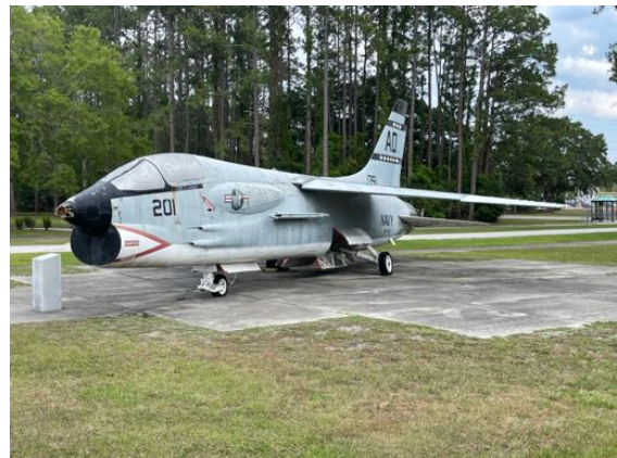
The lack of ventral fins indicate this is an F-8A
