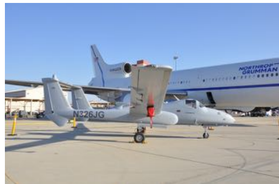
Northrop Grumman Firebird. This is an "optionally-piloted" aircraft, able to be operated as a manned aircraft or UAV. It's powered with a reciprocating engine.
