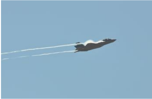
There was just enough humidity for some cool condensation in areas of low pressure. Here, the F-35 pulls up from a simulated attack run.
