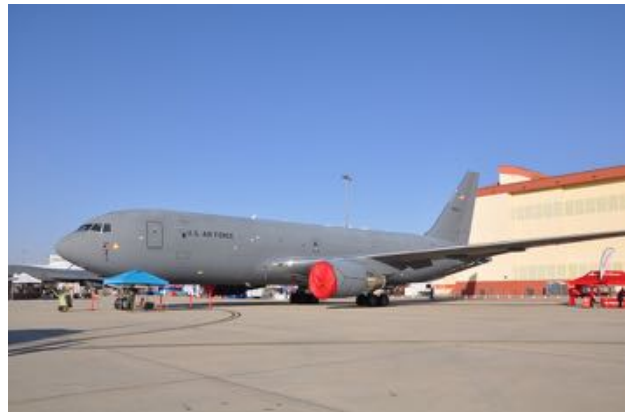
Boeing KC-46. This was the winner of the re-compete. Pentagon official Darlene Druyun was found to have 'cooked the books' in Boeing's favor and sentenced to prison. A 767-200, the KC-46 has had a protracted and troublesome development, including a boom system initially incapable of fueling large aircraft.
