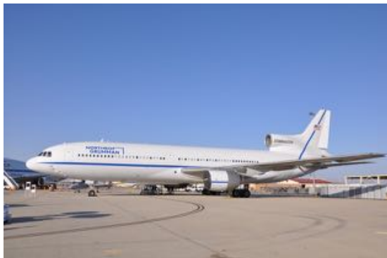
Northrop Grumman /OSC L-1011 "Stargazer" Used as a launch platform for the OSC Pegasus rocket. This is the last flying L-1011 in the world.
