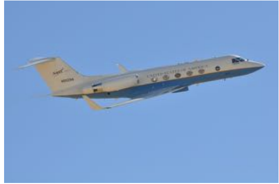
NASA Gulfstream C-20A. The pylon under the fuselage normally carries an earth-sensing synthetic aperture radar pod
