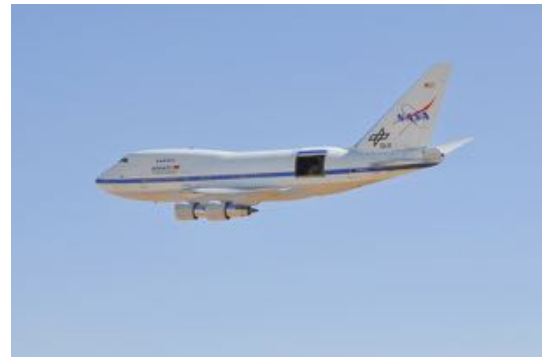
NASA 747SP SOFIA infrared observatory. This was the final public flight of SOFIA, as the program has been terminated following the successful launch of the James Webb Telescope. Here, SOFIA makes a pass with the telescope cavity door open, revealing the German-made 5-meter telescope.
