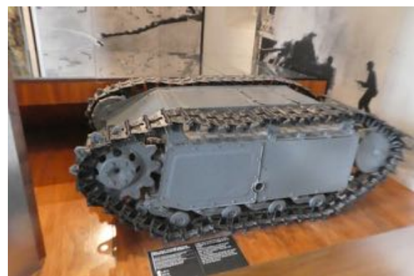
Panzer "Goliath" remote control tank. These were often packed with explosives and used as anti-tank weapons, and were not very successful. Tamiya has a kit with some very nice figures
