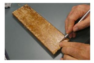
Tom then uses a sharp X-acto blade to trim the filament against a hard surface to the desired length of the antenna.
