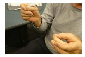
The speed which you pull the sprue determines the thickness of the filament – the faster you pull, the thinner the filament. However, if you pull too fast, you can break the filament.
