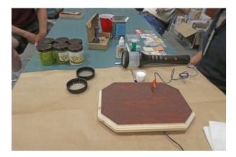
Rich applies water-based white glue to the base. The base has a nail inserted into it, which is attached to a lead on the applicator. This applies a charge to the conductive glue.
