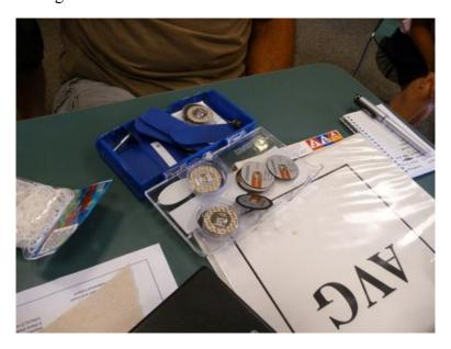
This is a new system from Dremel called EZ-Lock. It has a quick-change feature that allows you change out the wheel on the spindle with just a quick turn, instead of messing with a tiny screw. These are about \$12 to 15 a set at places like Home Depot and Lowe's.
