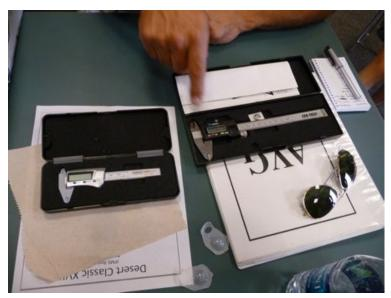
What the heck do I need a set of digital calipers for, you might ask yourself. Well, how about transferring dimensions? Or measuring a rigging span for a biplane. I know you can think of more, and they have uses outside of modeling. The small ones on the left are \$16 from Micro-Mark, while the larger set is \$15 from Harbor Freight. I have a nearly identical set that I use at work and they work great.
